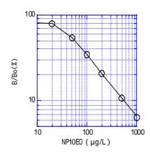
This test kit has a wide detection range between 0.02mg/ and 1mg/L.
